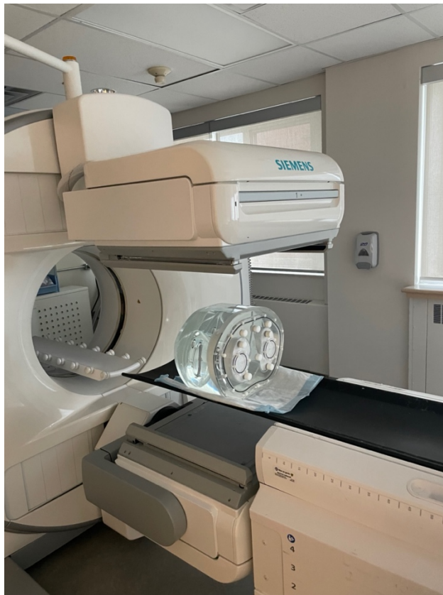
Figure 4.6- Imaging of the Data Spectrum Anthropomorphic Torso Phantom inside the Siemens Intevo Bold SPECT/CT. The phantom, tailored with dimensions of 45×33 cm, represents larger patient sizes and anatomical structures pertinent to nuclear lung scans.
